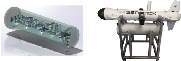
Figure 3. Layout definition to minimize dead volumes. The system is designed to be embedded on an Autonomous Underwater Vehicle (AUV).
